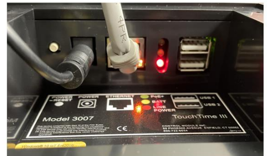
From left to right: Power/Reset button, AC power in, Ethernet in, status lights, (2) USB 2.0 ports To reset the clock, unplug the power and Ethernet cables. Then hold the Power/Reset button for 10 seconds, until the screen turns blank.
